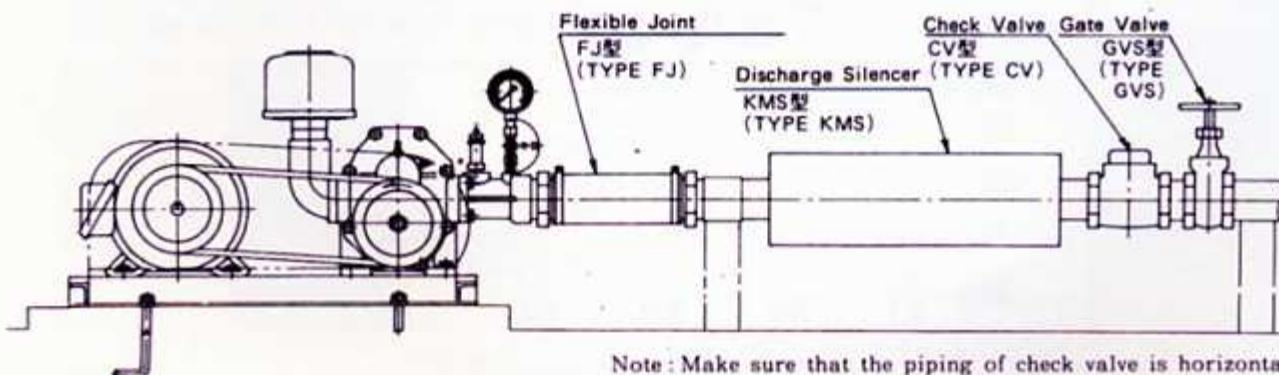
Note: Make sure that the piping of check valve is horizontal.
