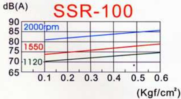
NOISE LEVEL dB[A] Machine Side 1.0m
